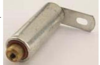
A simpler way of checking if it's a bad condenser is to remove the distributor cap, body and rotor. Make sure the points are closed. Turn the ignition switch on and place the high tension wire (from centre of coil) about one-half inch from any convenient ground on the engine. Push points open with a screwdriver then close. The spark should jump the gap with a sharp crack and a straight line. The spark should have a blue tinge.
