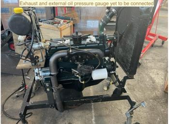
starter motor with plenty of enthusiasm, needed for the tight engine. We set up the distributor and a standard Zenith Carb and inlet manifold. After setting the timing pin into the notch in the camshaft gear to get No1 'top-dead-centre' we used a NuRex timing gauge to set the static timing to 4 degrees after TDC, having already set the contact breaker and spark plug gaps to factory spec.
